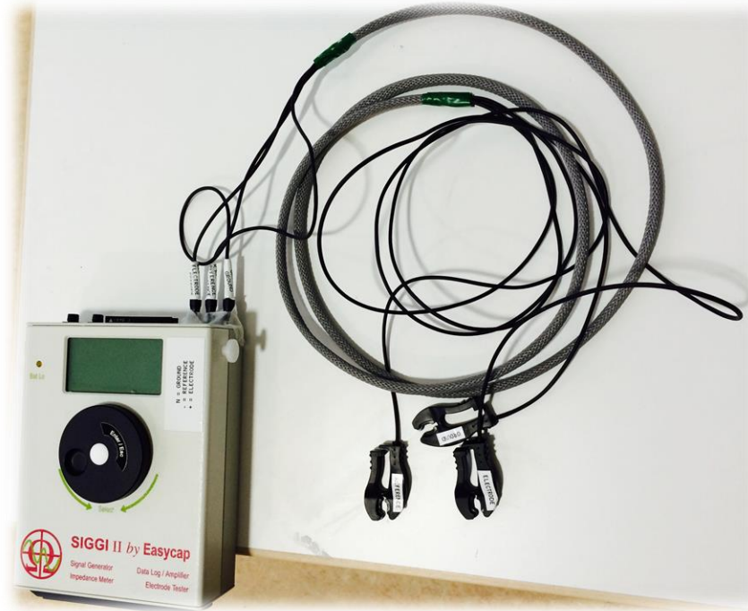
Impedance meter with cables
